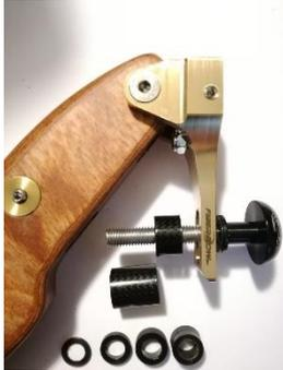
Repeat the measurement sequence for the opposite side and replace the black rubber with the spacers supplied trying to match the measurement made.
