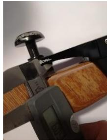
Before removing the adjusting screw, measure the distance between the cradle and the riser surface at a specific point.
