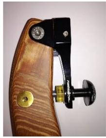
Replace the black rubber that pushes the cradle with the nylon washer and the M8 brass nut supplied.
